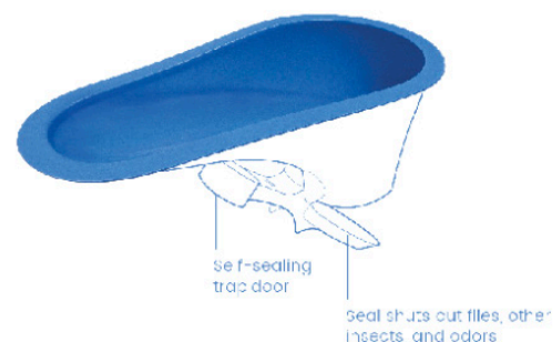
The SATO conventional toilet pan mechanism.
